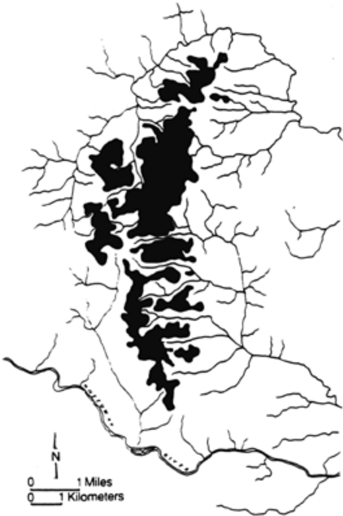
Figure 7 – The Old Hickory heavy-mineral deposit, located in Sussex and Dinwiddie counties, Virginia, is an example of a heavy-mineral deposit that has been subjected to erosion. Dark areas are the locations containing commercial mineralization. Narrow linear features are modern creeks and drainages responsible for the erosion.
