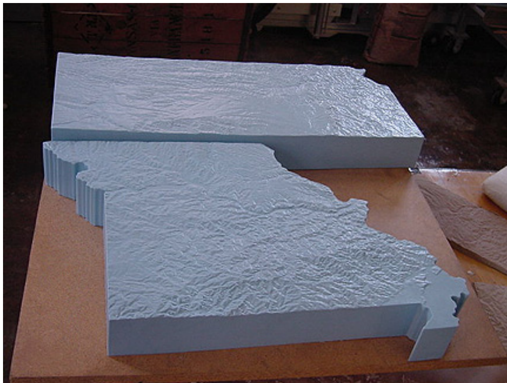
Silicone rubber casts, made from the same polyurthane rubber molds used to cast the plaster Kansas and Missouri topographical models. These silicone casts will be used to create new plaster molds, which will then be used for casting a series of ceramic topographical models.
