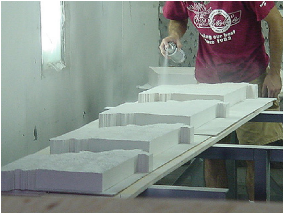
Once the plaster and cement mixture has completely cured, the topographical models are sprayed with a white primer. Summer 2003.
