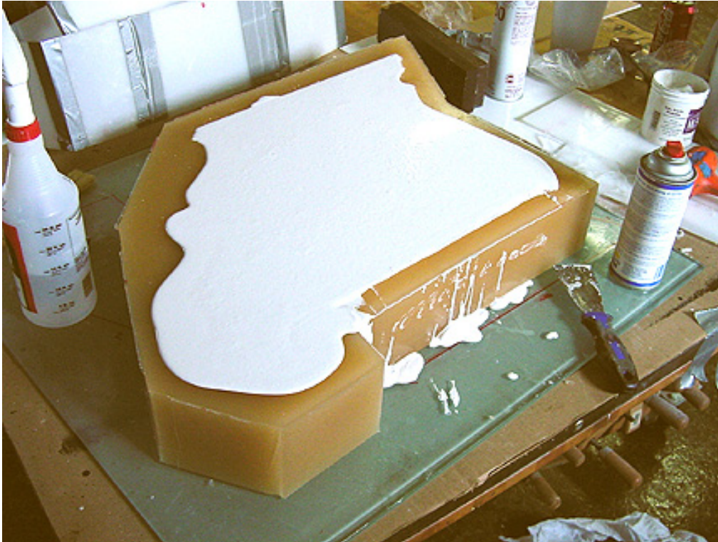
Once the polyurethane rubber mold has cured, a liquid mixture of plaster and cement (Hydrostone) is poured into it, to creating the final 3-D topographical model. Summer 2003.
