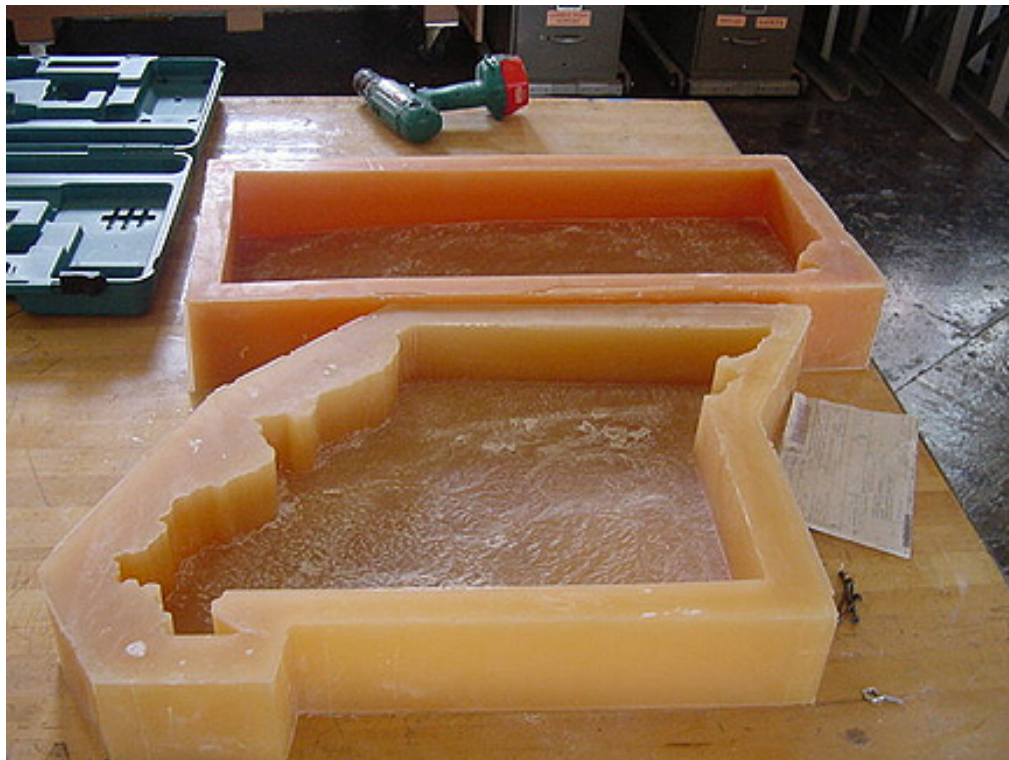
The two polyurethane rubber molds used to make the topographical models of Missouri and Kansas. The models are being donated to regional historical society museums in both states. Grandarts workshop, Summer 2003..
