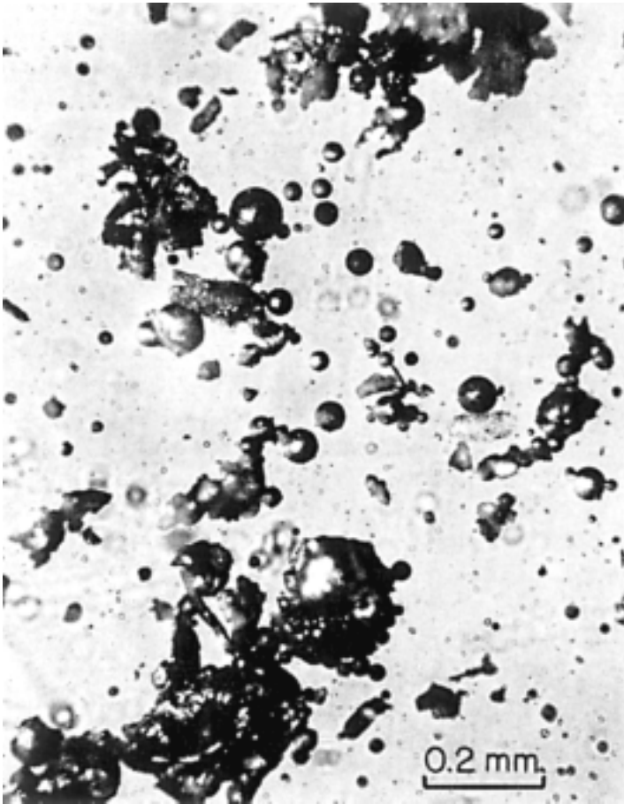
Figure 2: Photomicrograph of grains from iron fulgurite showing spheres, filaments, and irregular masses of iron.
