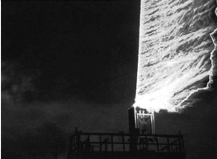
A wind-blown triggered lightning strike, staged at the Camp Blanding lightning research facility. More than 30 triggered lightning strikes are staged there each year, allowing scientists to study how lightning strikes affect power lines, airport runways, home appliances, and other systems.
