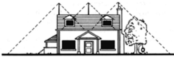
Figure 2.2: (a) A house protected by a single lightning rod having an assumed 45°-angle cone of protection - that is, the height of the rod is  $H$  and the base area assumed to be safe from a lightning strike has a radius  $H$ . (b) The same house protected by a lightning rod system consisting of three smaller rods, each assumed to provide a 45°-angle cone of protection.
