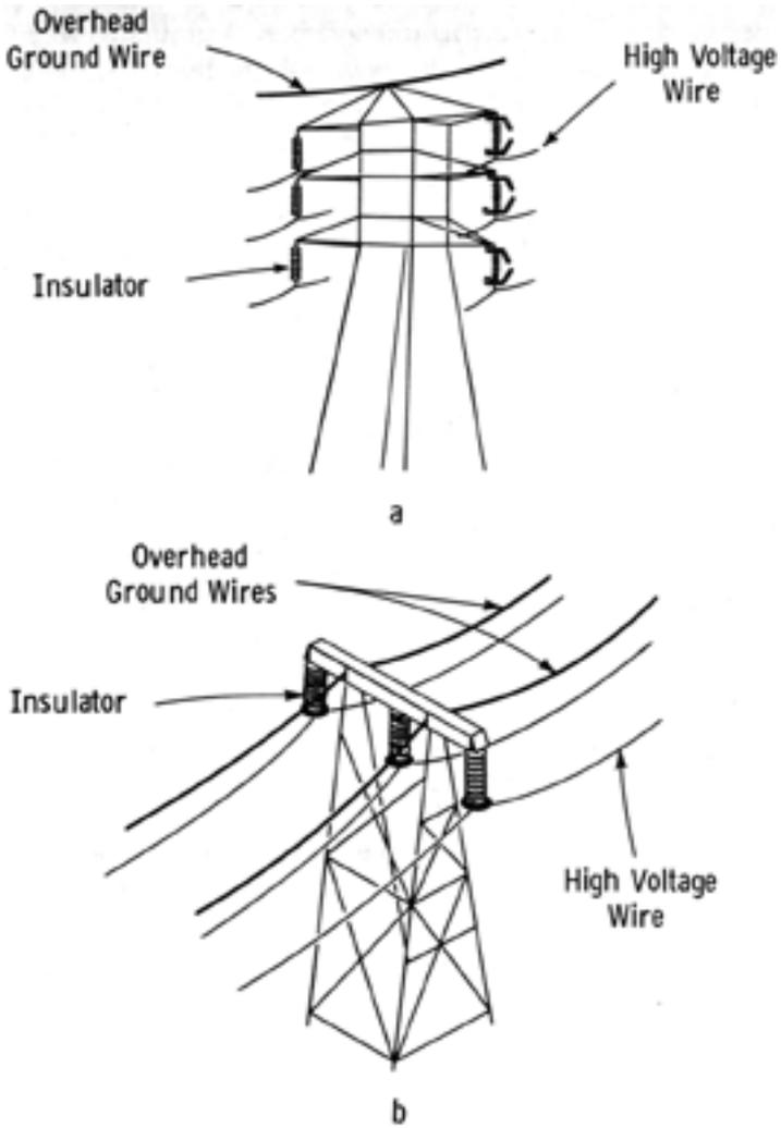
Figure 2.3: Use of overhead ground wires to protect high voltage transmission lines from lightning. Each of the high voltage wires is supported by the bottom of an insulator. Ground wires are attached to the metal transmission line towers which are well grounded. Drawings are not to scale. (a) A typical 132,000 volt line. (b) A typical 220,000 volt line.
