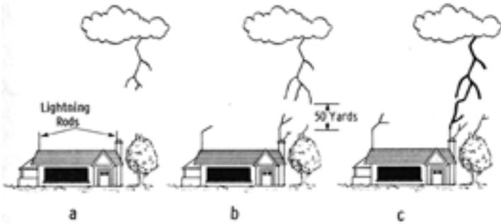
Figure 2.1: Final stages of a strike to a lightning rod. The time interval between B and A and between C and B is about  $1/5000$  second. The lightning channel becomes very bright (view C) immediately after the upward-traveling spark connects with the downward-moving lightning. Drawings are not to scale.
