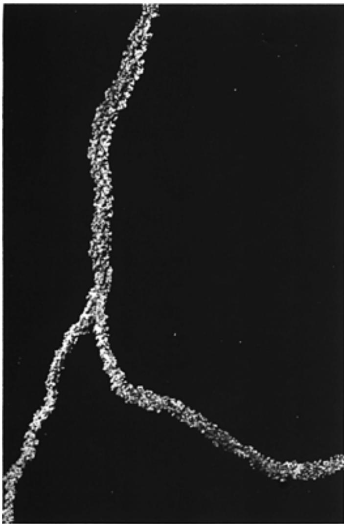
A portion of a 5 1/2 foot recovered section of a fulgurite. Diameter is 1 inch. Branching is a permanent record of the course of the discharge. Found in Oceana County, Michigan. Photo and specimen, Terry Huizing.
