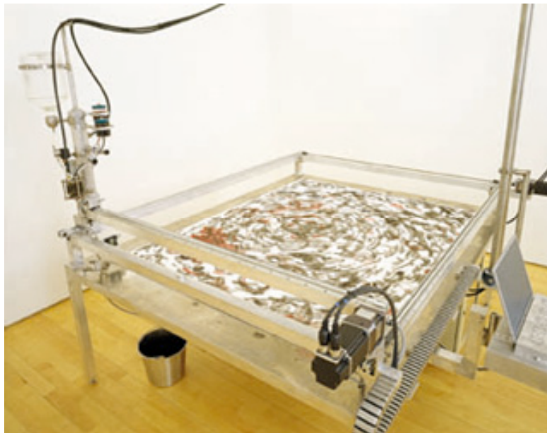
Drawing Machine , 2000. Aluminum, stainless steel, glass, valves, servo monitors, track, computer custom hardware, ink, paper. 90" x 94" x 90".
