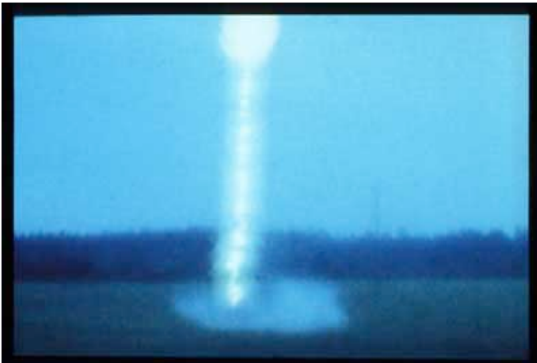
Lightning strike that formed the fulgurite, at the University of Florida's International Lightning Research Facility at Camp Blanding, Florida. Sixteen millimeter frame, shot at 500 frames per second.
