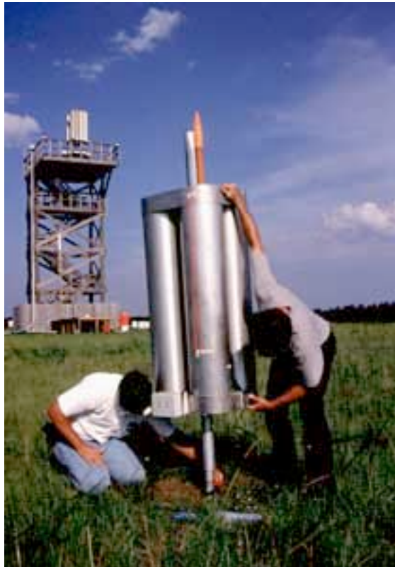
Allan McCollum at the International Facility for Lightning research, preparing rocket used to trigger lightning, at Camp Blanding, Florida. 1997.
